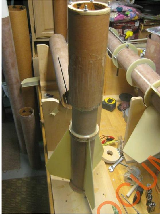
Figure 19 – Booster airframe ready to be installed.
